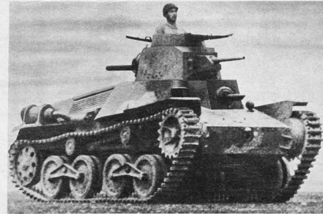
Triple armament of 2595 includes a 37-mm. gun in the turret, a machine gun in the right rear of turret, another in the left front of hull. The guns cannot fire simultaneously. Later models may mount a 47-mm. cannon. Turret is roughly conical with cupola atop. Hull has angular bow.
